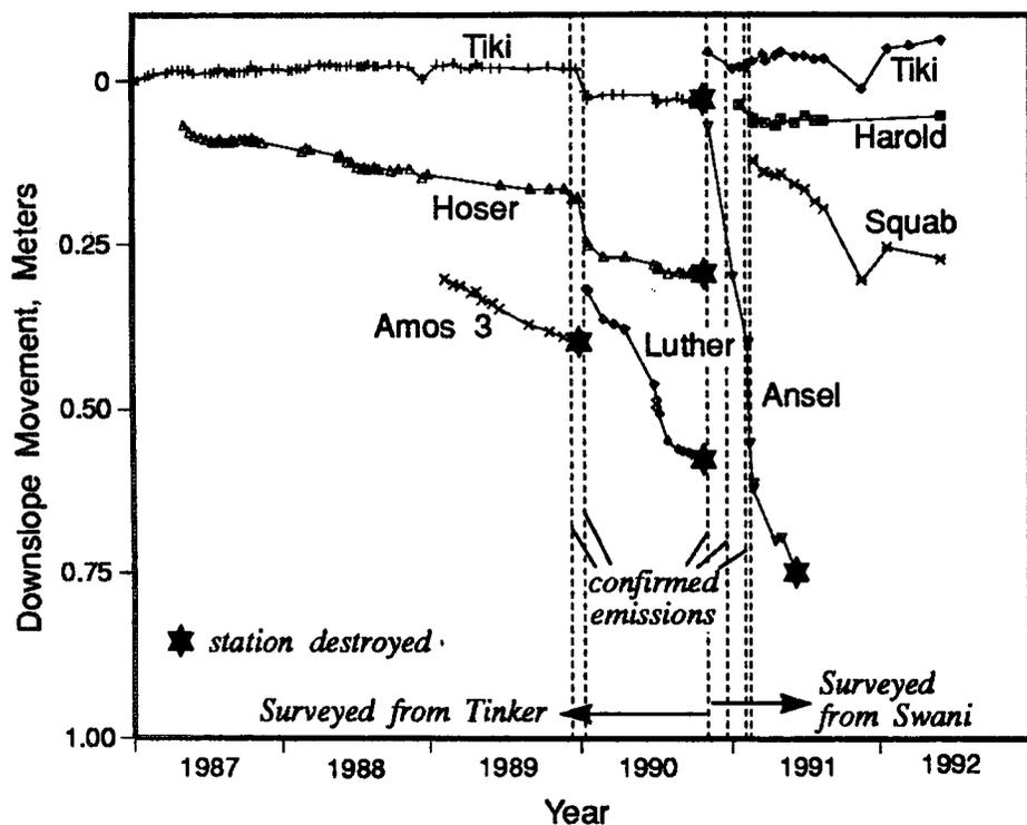
**Figure 10.** Changes in slope distance versus time, measured from points north of the dome to geodetic stations on the north side of the dome. Locations of geodetic stations are shown in Figure 3. Before 5 November 1990, stations were surveyed from the point Tinker, near the north base of the dome. After 5 November 1990, they were surveyed from a station (Swani) ~1.8 km north of the dome.
